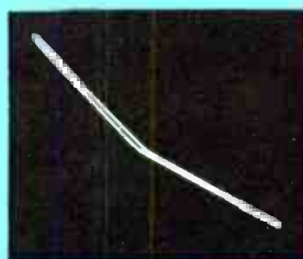
(D) A PNP germanium transistor with the emitter connected to G, the base to H through a 6.8K-ohm resistor, and a 6.8K resistor in parallel with the base and emitter. The waveform approaches that of a pure resistance, but the diode corner is still visible.
